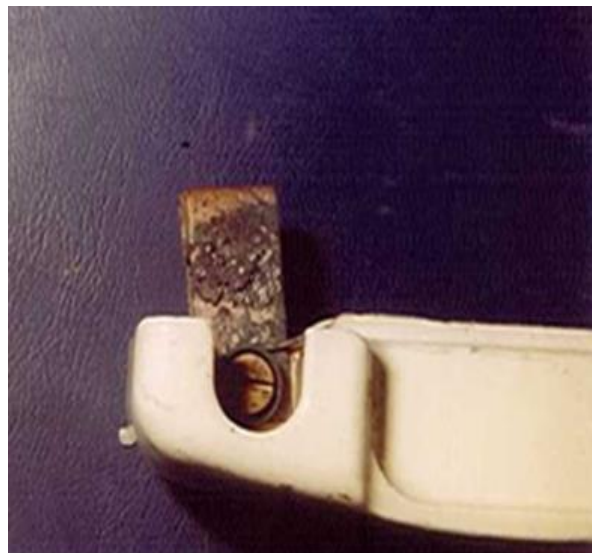
Pitted blade, due to making poor contact
